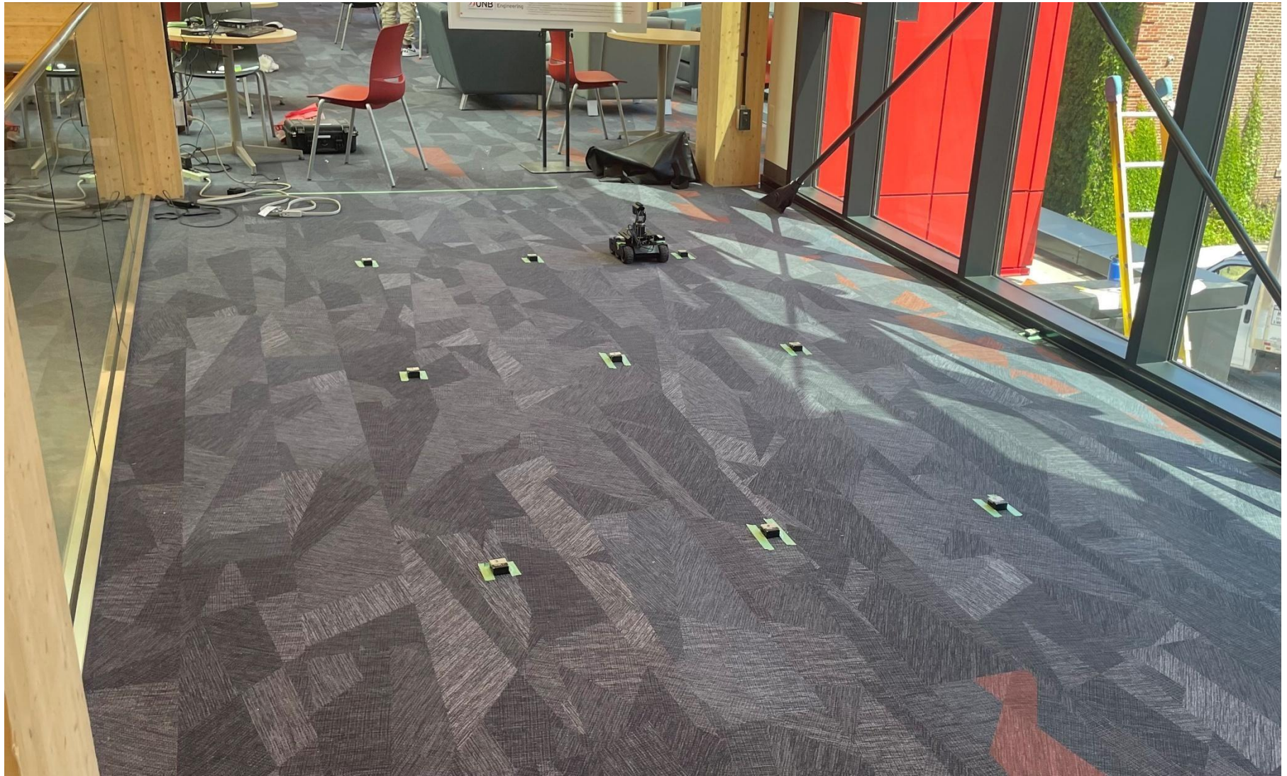
Figure 4: UGV Rover Platform Mounted with Accelerometers and Compared to Stationary Accelerometers
